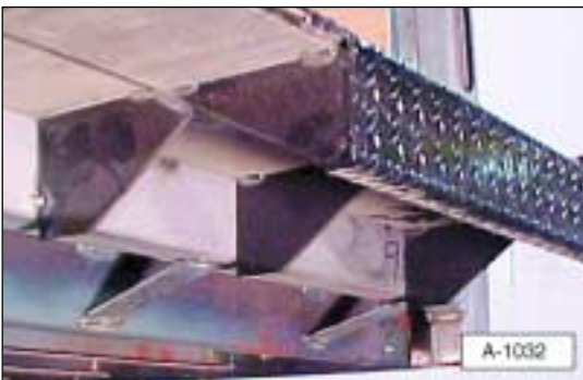
Illustration 4c. Tack weld floor extension brackets.
