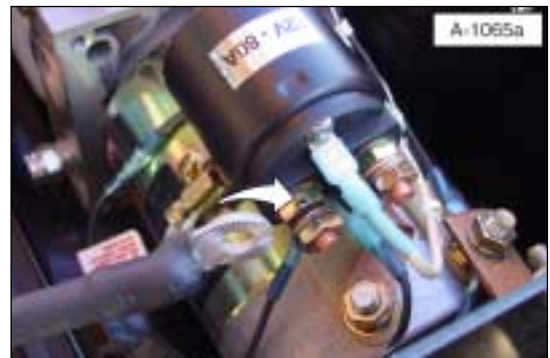
Illustration 8c. Connect power cable to motor solenoid.
