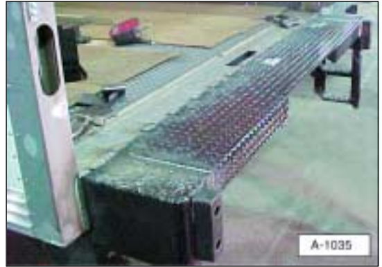
Illustration 20c. Correctly welded floor extension and dock bumper corners.
