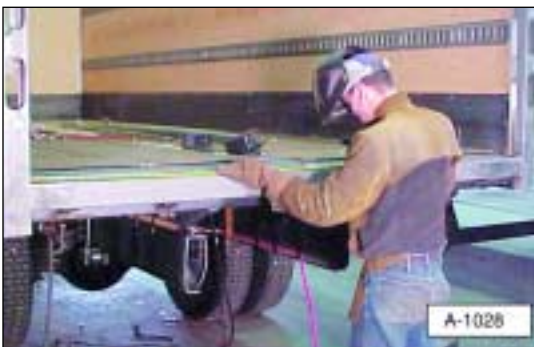
Illustration 3. Find and mark the center of truck's rear sill.
