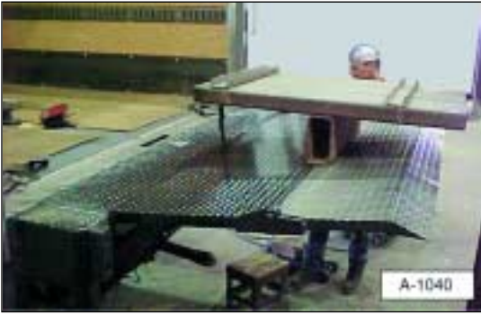
Illustration 5b. Align the center mark of the liftgate platform with the center mark on the floor extension.
