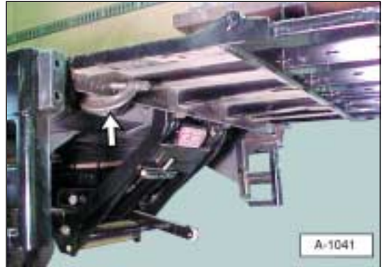
Illustration 6a. Clamp liftgate onto floor extension.
